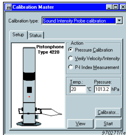
Fig. 6 Calibration Master showing the setup for calibrating a sound intensity probe
